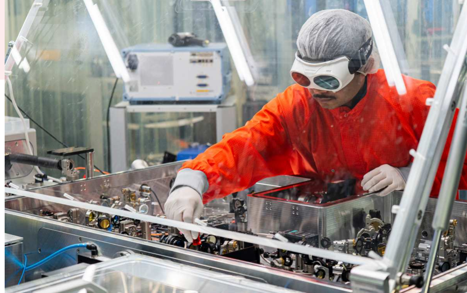
Abhijit Maity performs final checks on the recently upgraded Infrasampler 1.5 system before it is transported to the new CMF laboratory in Szeged. After reinstallation, it will be used to determine the electric-field molecular fingerprint of thousands of H4H samples. Photo: Thorsten Naeser
